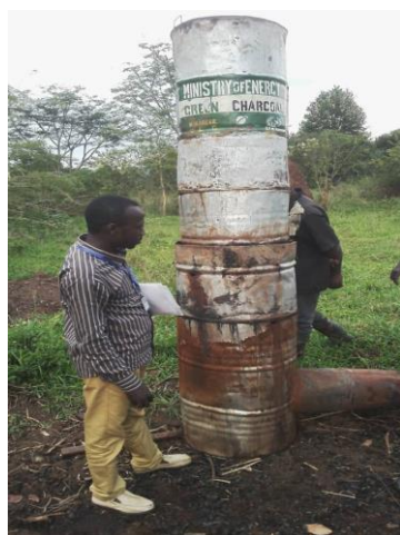
Figure 2: Green charcoal processing using collapsible kiln, in Kapeeka Sub-county, Nakaseke District
